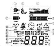
voltage range. When the sensitivity is increased, the UPS will switch to Battery Mode with less input power variation
